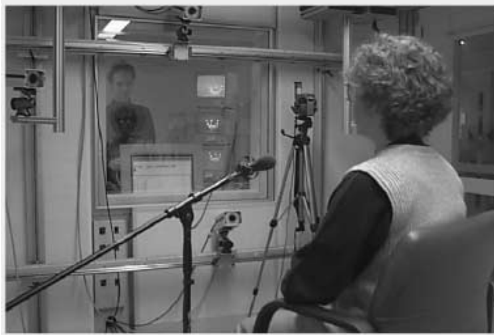
Figure 1: The recording setup. The person whose facial motion is to be recorded is seated in a chair. Four infrared cameras (one is hidden behind the person), an ordinary video camera, and a microphone are pointed at the person's face. In front of the person is a screen showing the text and emotion to be read/acted by the person.
